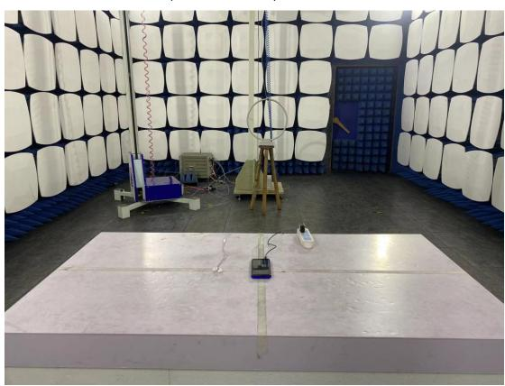
3. Radiated emission (9KHz-30MHz)
