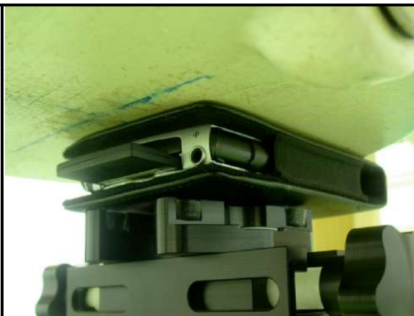
B: The front of the EUT face to the phantom with 14mm-separation distance.
