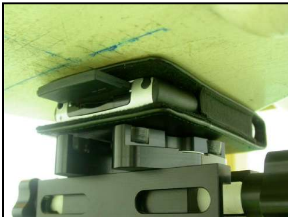
A: The bottom of the EUT face to the phantom with 7mm-separation distance.
