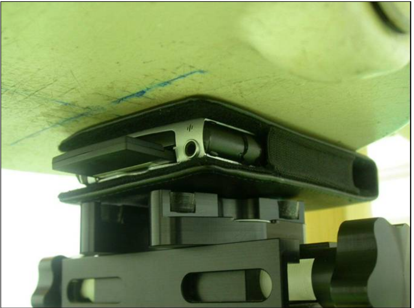
The front of the EUT to the flat phantom distance 14 mm
