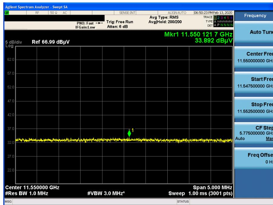
**Unwanted Emissions (Radiated) Test Plot \_ MN: ADC40S2AN**
