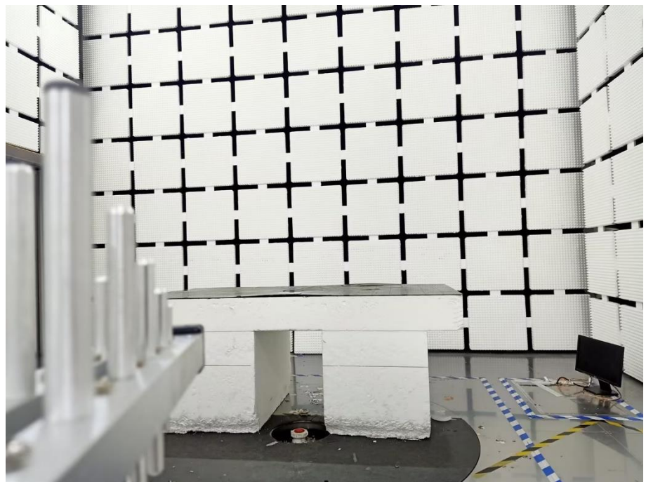
Radiation Emission Test Setup (30MHz to 1GHz)
