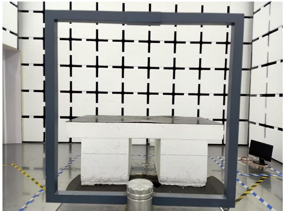
Radiation Emission Test Setup (Below 30MHz)
