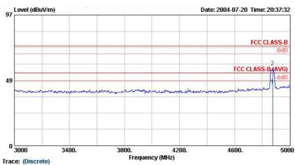
03CH06 FCC CLASS-B 3m HF-HORN AH-118 VERTICAL 802.11a/b/g Access Point Condition
