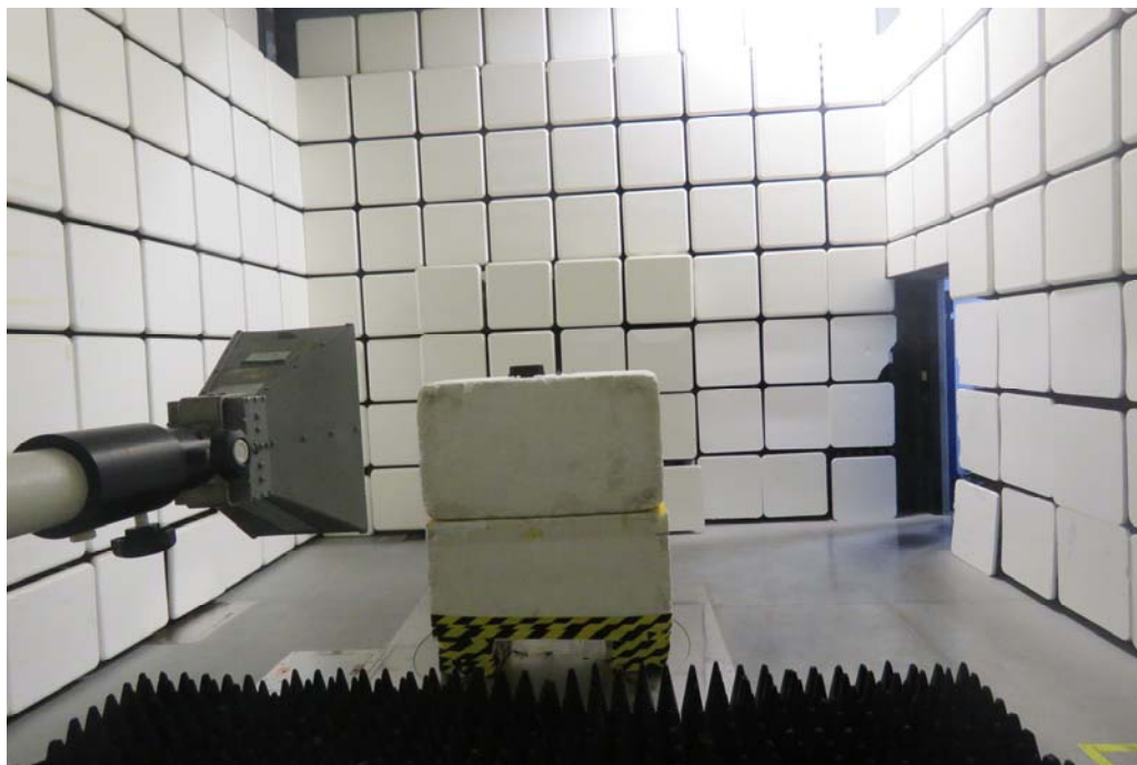
Picture 1: Radiated Spurious Emissions Test setup
