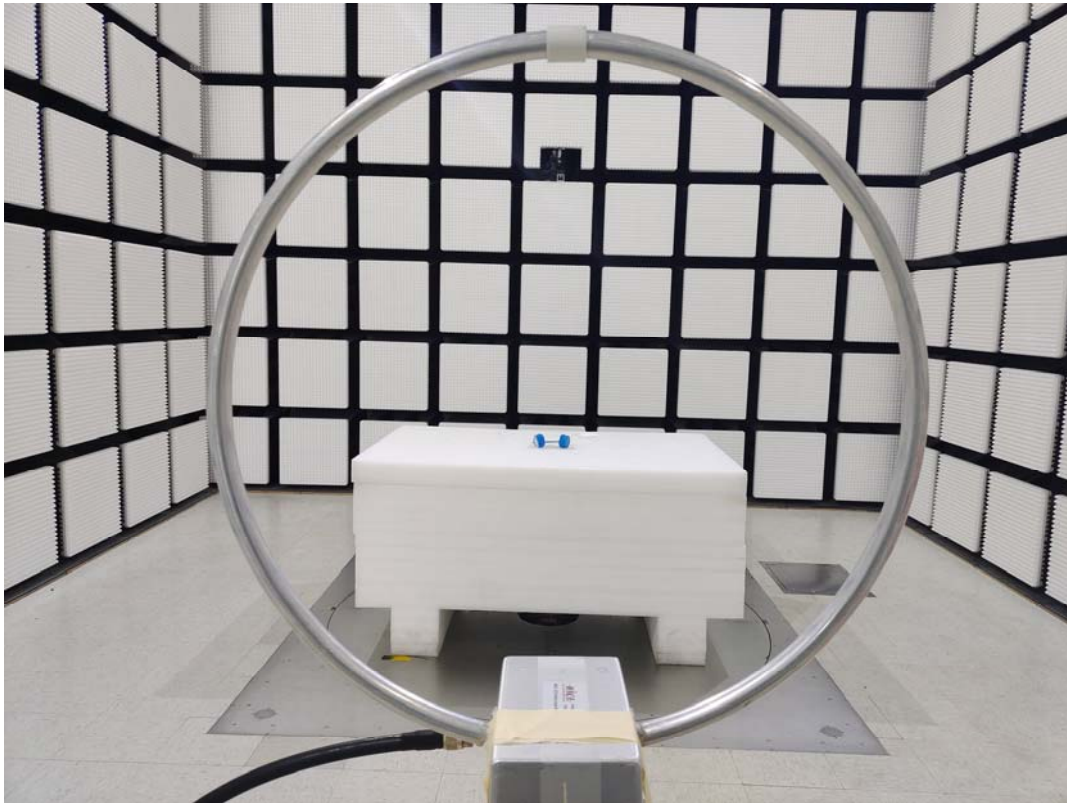
9kHz to 30MHz_Radiated Emission_Perpendicular
