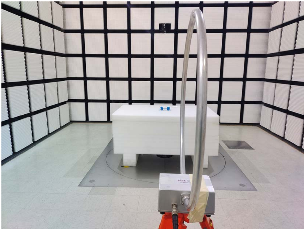
9kHz to 30MHz_Radiated Emission_Perpendicular
