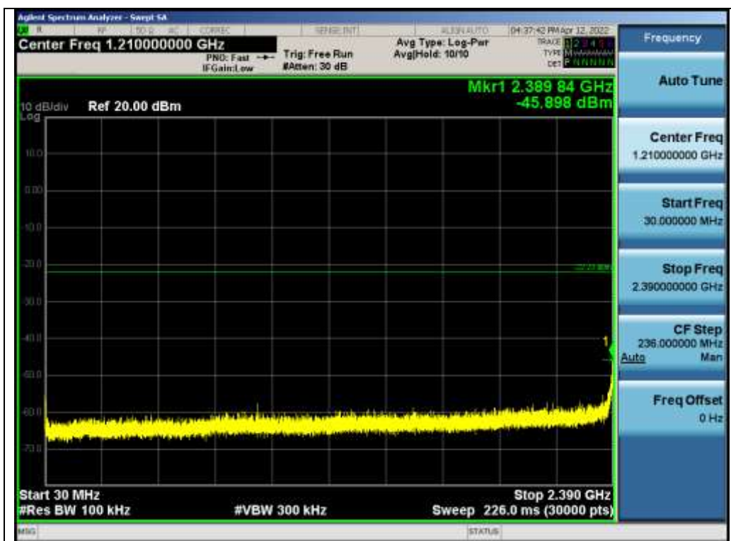
Test_Graph_802.11n20_ANT1_2412_MCS0_Lower Band Emissions
