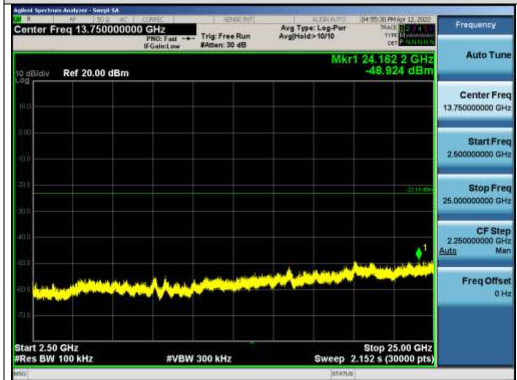
Test_Graph_802.11n20_ANT1_2462_MCS0_Higher Band Emissions
