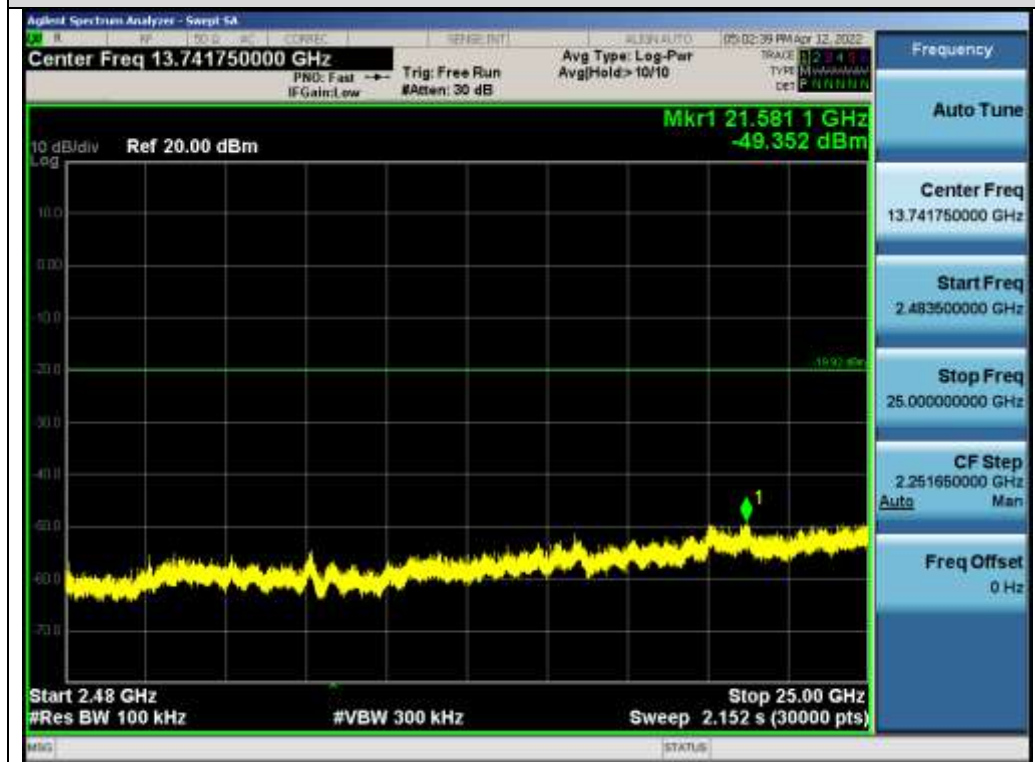
Test_Graph_802.11g_ANT1_2412_6Mbps_Higher Band Emissions
