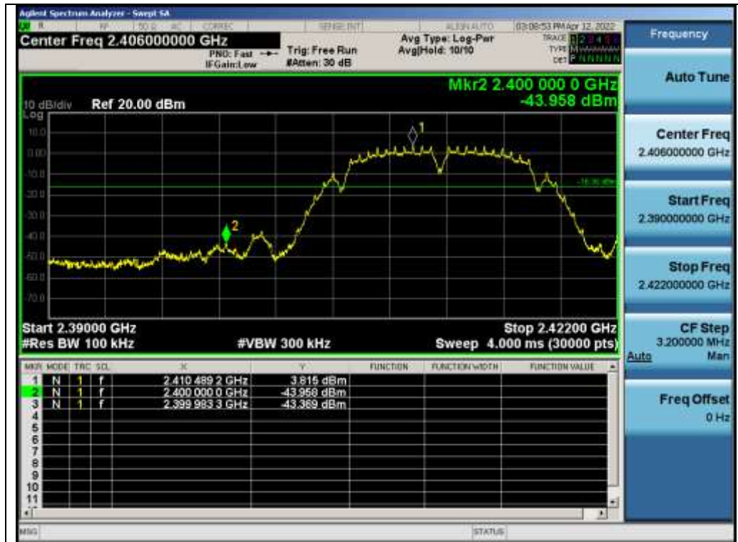
Test_Graph_802.11b_ANT1_2412_1Mbps_Lower Band Edge Emissions
