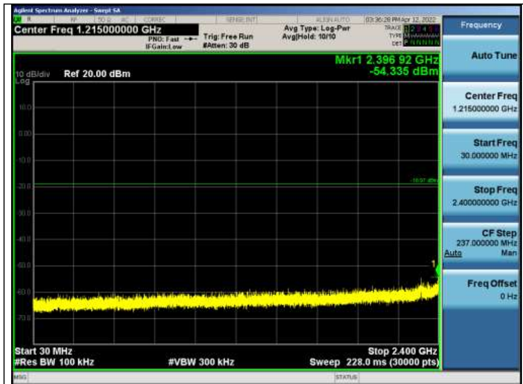
Test_Graph_802.11g_ANT1_2462_6Mbps_Lower Band Emissions
