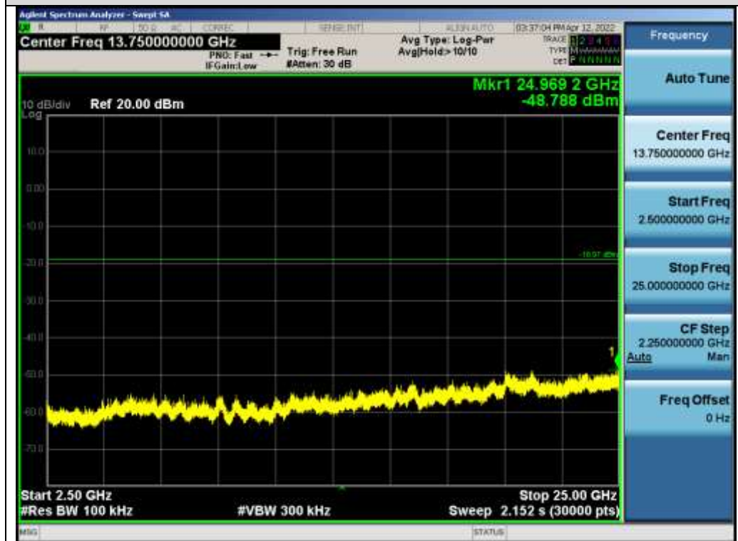
Test_Graph_802.11g_ANT1_2462_6Mbps_Higher Band Emissions
