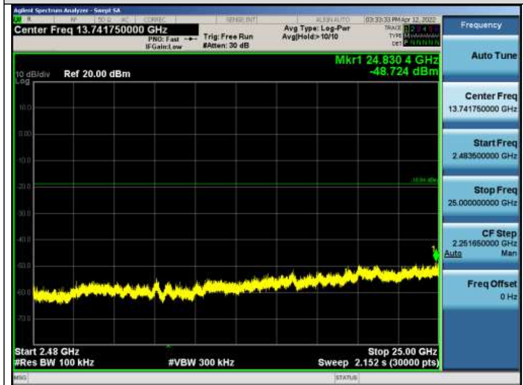
Test_Graph_802.11g_ANT1_2437_6Mbps_Higher Band Emissions
