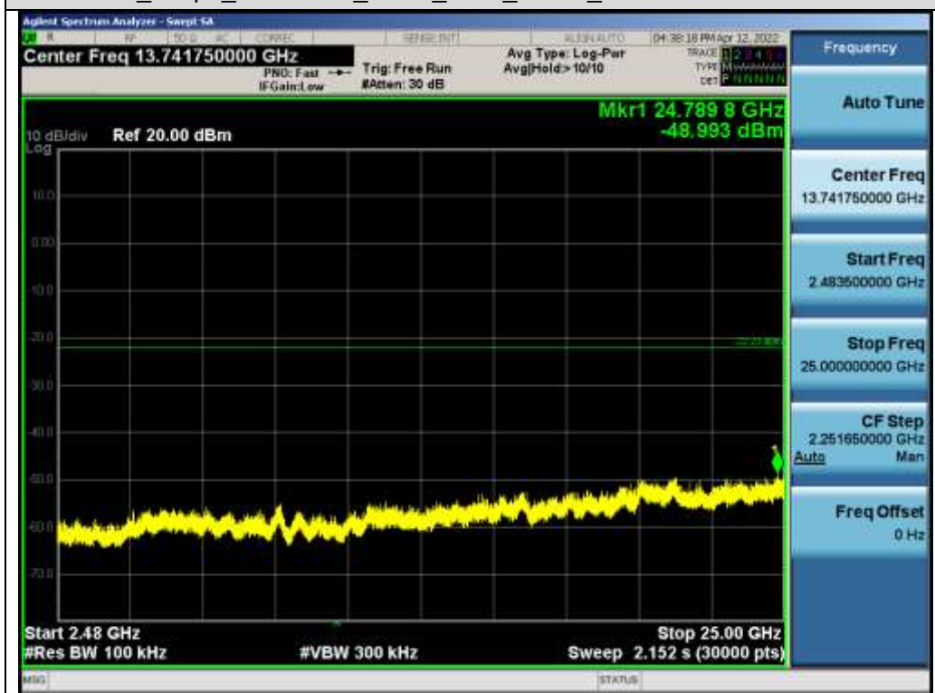
Test_Graph_802.11n20_ANT1_2412_MCS0_Higher Band Emissions
