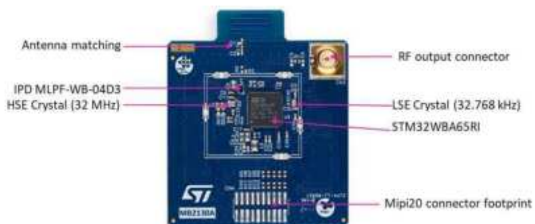
Figure 3 MB2130A PCB top view
