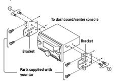
When mounting this unit to the preinstalled brackets of your car, use the mounting screws ① in the appropriate screw holes based on your car: T for TOYOTA and N for NISSAN.
