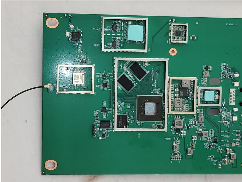
**Photograph 5: PCB Bottom (Shields Removed)**
