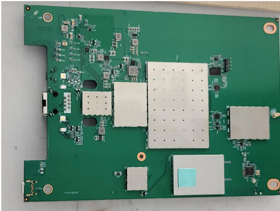
**Photograph 4: PCB Bottom (Shields in place)**
