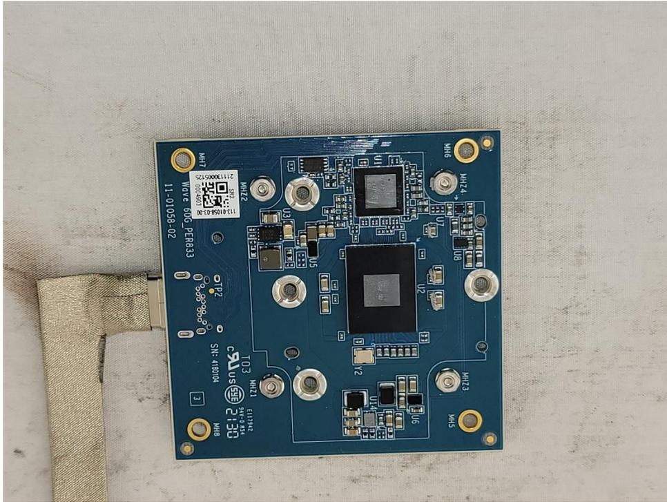
**Photograph 7: 60GHz Antenna and module Bottom**
