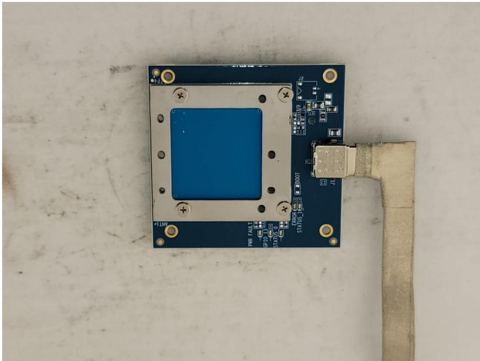
**Photograph 6: 60GHz Antenna and module Top**
