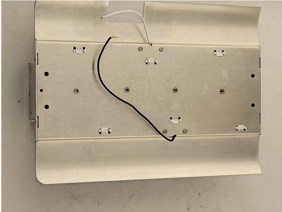
**Photograph 9: 5GHz Antenna Bottom**
