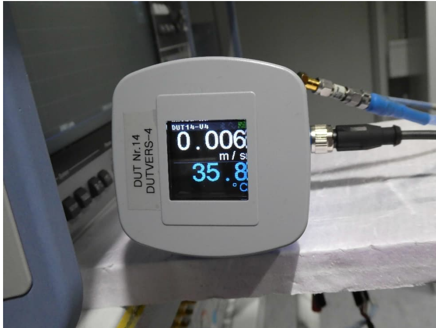
Test setup conducted @ antenna port Preliminary and final measurement 9 kHz – 26.5 GHz
