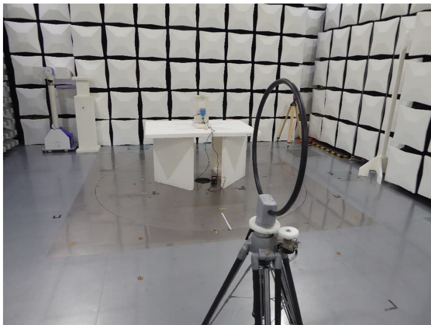
EUT Position 1 / Antenna Position 2 Test setup semi-anechoic chamber M276 Preliminary measurement
