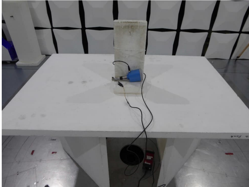
EUT Position 3 Test setup semi-anechoic chamber M276 Preliminary measurement
