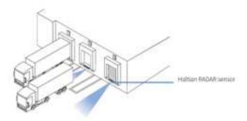
Please check that the installation spot is not impacted by any moving mechanisms in the loading dock during its operation. The RADAR should be installed in a location where it will not be hit or damaged by a truck backing up or approaching the loading dock.
