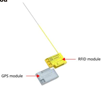
Combine RFID module and GPS module together.
