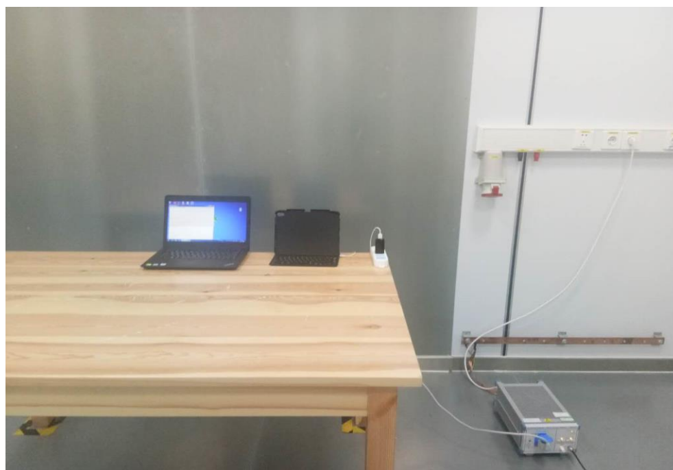
Fig. 4 Power line conducted emission setup photo
