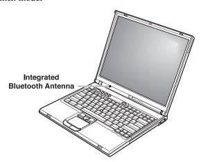
**Note:** The antenna of the model BMDC200 is located on the left side of the computer lid in the ThinkPad T40 Series 14-inch model, or on the bottom of the computer lid in the ThinkPad T40 Series 15-inch model. Transmitted energy from the *Bluetooth* device is very low compared to other RF devices. Therefore a 20 cm separation from the *Bluetooth* antenna is not required.
