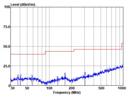
Antenna Polarity :VERTICAL EUT/Project :7211CR
