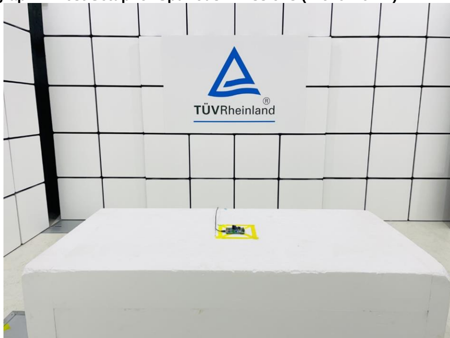
Photograph 2: Test Setup for Spurious Emissions (Front View 2)
