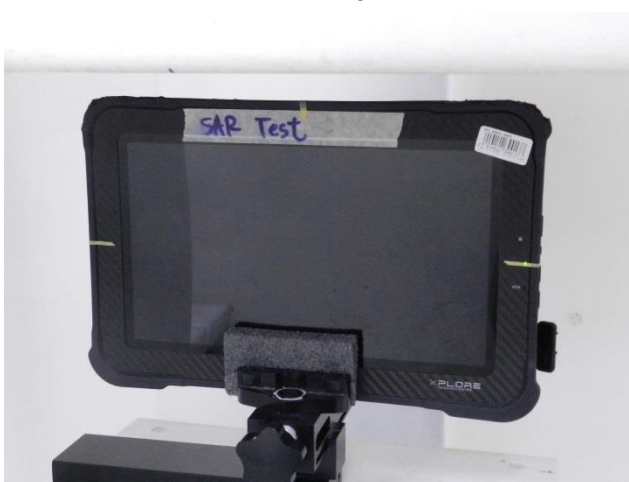
Edge1, Test Separation 1.5 cm
