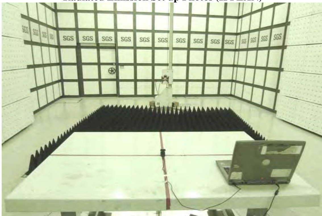
Radiated Emission Set up Photos (H PLAN)
