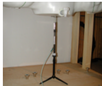
Figure 12.1 Dipole Validation Test Setup
