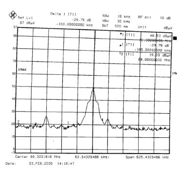
Note: The field strength of any emissions radiated on any frequency outside of the specified 200 kHz band is below the general radiated emission limits in §15.209.
