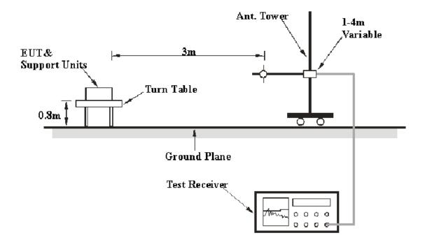
The radiated emission tests were performed in the 3-meter chamber, using the setup accordance with the ANSI C63.4 - 2003. The specification used was the FCC 15.209 and 15 .239 Limits.
