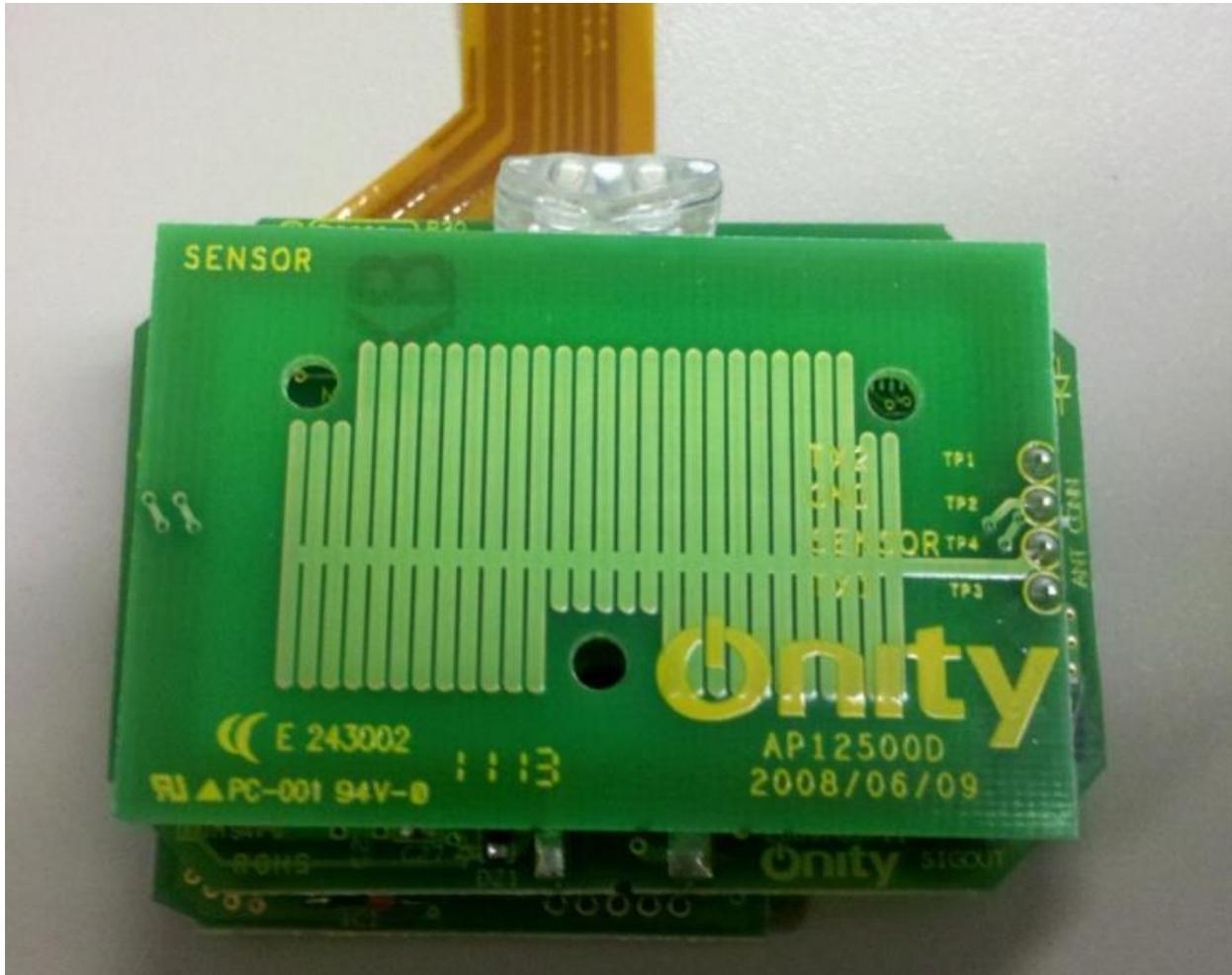
Figure 2. The RFID antenna mounted to the top of its other RFID PCBs.
