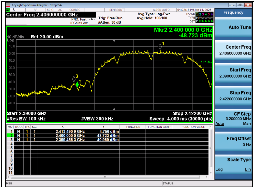
Test_Graph_802.11b_Chain A_2412_1Mbps_Lower Band Edge Emissions
