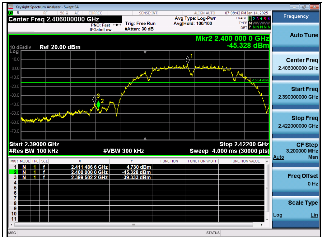
Test_Graph_802.11b_Chain B_2412_1Mbps_Lower Band Edge Emissions
