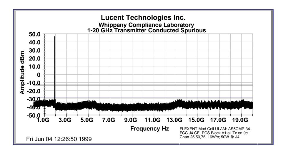
Conducted Spurious Measurement of Antenna Output Port When Transmitting in PCS Block A3, Three Carrier Configuration
