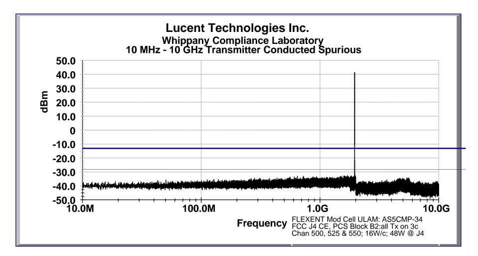
Conducted Spurious Measurement of Antenna Output Port When Transmitting in PCS Block B2, Three Carrier Configuration
