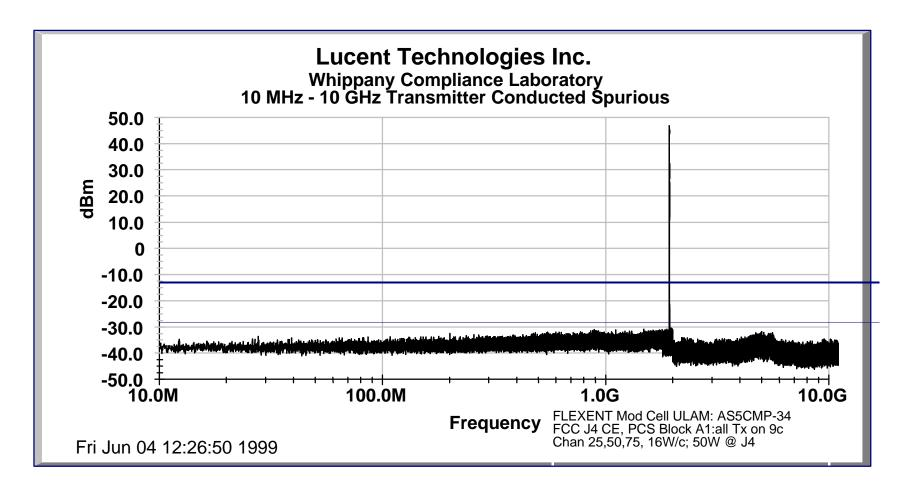
Conducted Spurious Measurement of Antenna Output Port When Transmitting in PCS Block A1, Three Carrier Configuration
