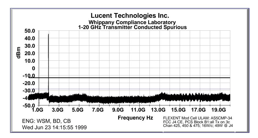
Conducted Spurious Measurement of Antenna Output Port When Transmitting in PCS Block B2, Three Carrier Configuration
