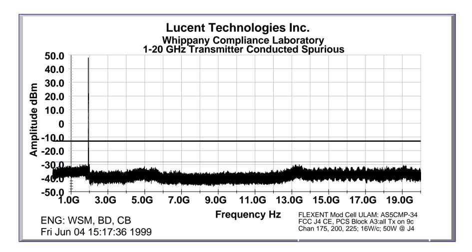
Conducted Spurious Measurement of Antenna Output Port When Transmitting in PCS Block B1, Three Carrier Configuration
