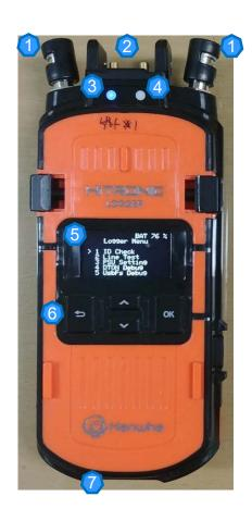
1) Binding Post : Connect detonators
