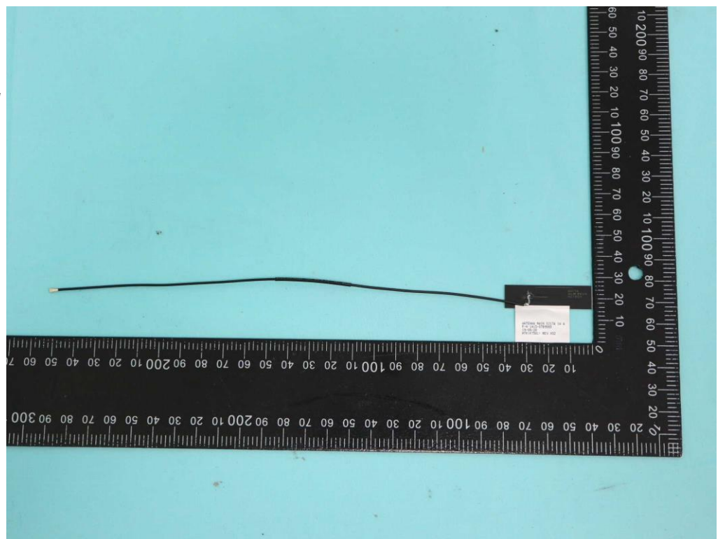
Antenna 1 (HIGH-TEK ELECTRONICS CO., LTD/ 0ACPG019003N)
