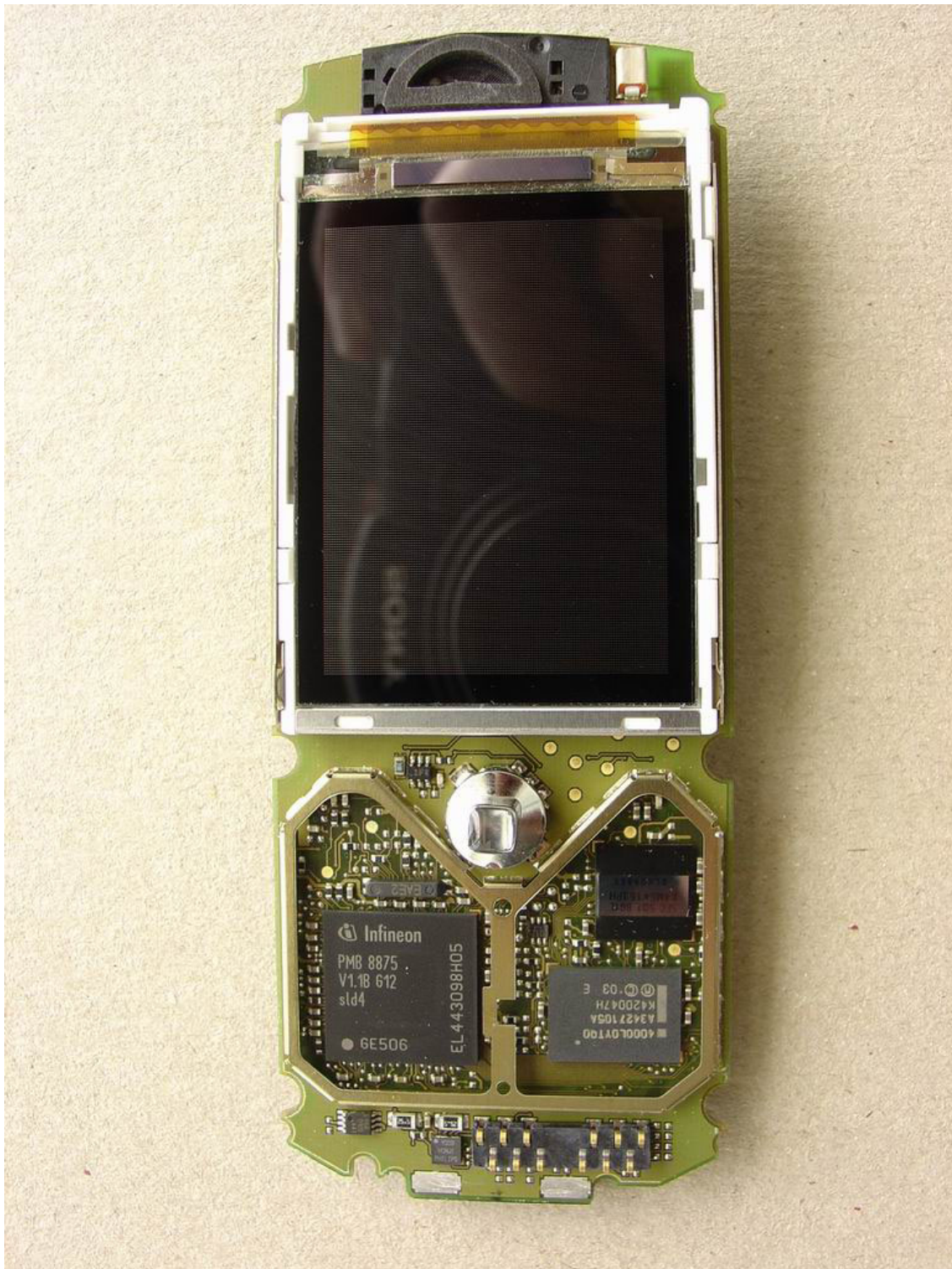
CX75 PCB Front View Shields Removed
