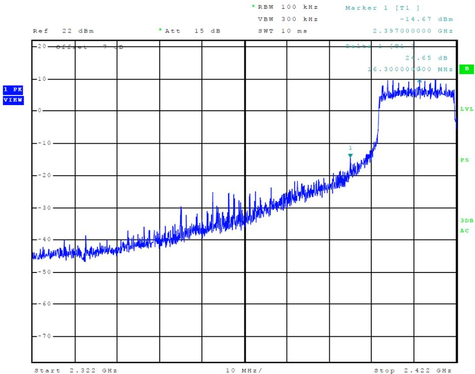
**Figure 10 Plot of Transmitter Low Band Edge (802.11n (40))**
