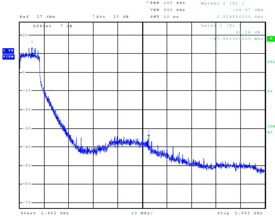
Figure 13 Plot of Transmitter High Band Edge (802.11n (20))
