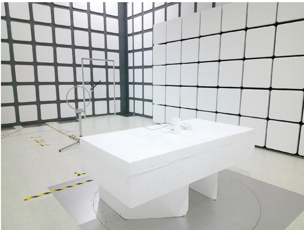
Description: Radiated Emission Test Setup for 30MHz~1GHz
