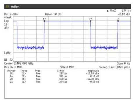
Duty Cycle = Ton / (Ton + Toff) =  $391[\mu s]$  /  $(391[\mu s] + 234[\mu s]) = <math>62.56[\%]$
