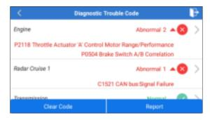
The system with fault codes will be displayed in red ( $\otimes$ ). The system with no fault codes will be displayed in green ( $\checkmark$ ).
