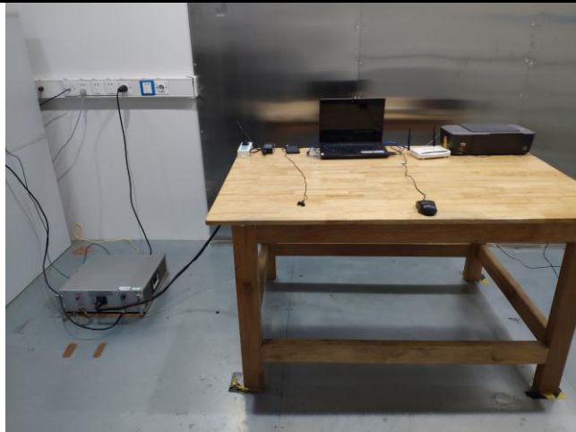
Conducted Emissions Test Setup – Front View
