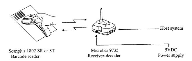
The user activates the Scanplus 1802 scanner by pressing on its trigger and aims the light beam at the barcode.
