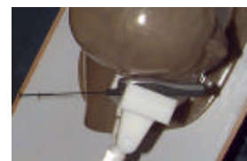
Fig. 14 Head SAR Test Setup
