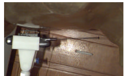
Figure 17. Body SAR Test Setup
