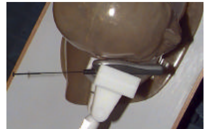
Figure 15. Head SAR Test Setup
