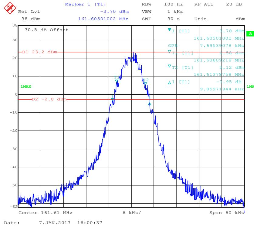
**Frequency 161.61 MHz: 99% Occupied & 26 dB Bandwidth with Low Power--- Part 22**
