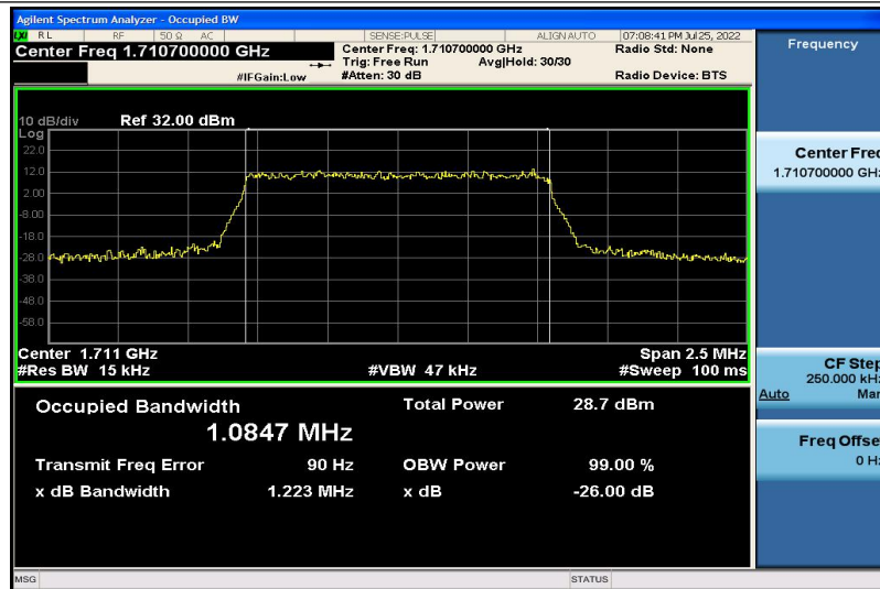
Band4-1.4MHz-QPSK-19957-6RB#0-1.0847
