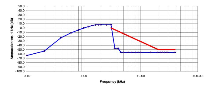
AUDIO FREQUENCY REPSONSE @ FCC 2.987(a) & 90.242b(8) Technisonic 800 FM Transceiver (12.5 kHz Channel Spacing)
