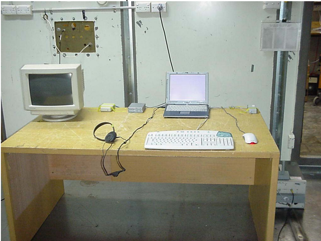
Conducted Emissions Test Setup
