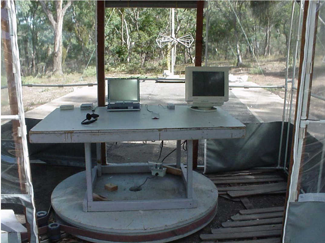
Radiated Emissions Test Setup (10 metre distance)
