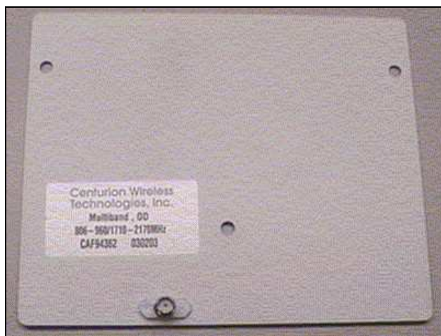
Figure B- 9: GSM Antenna
