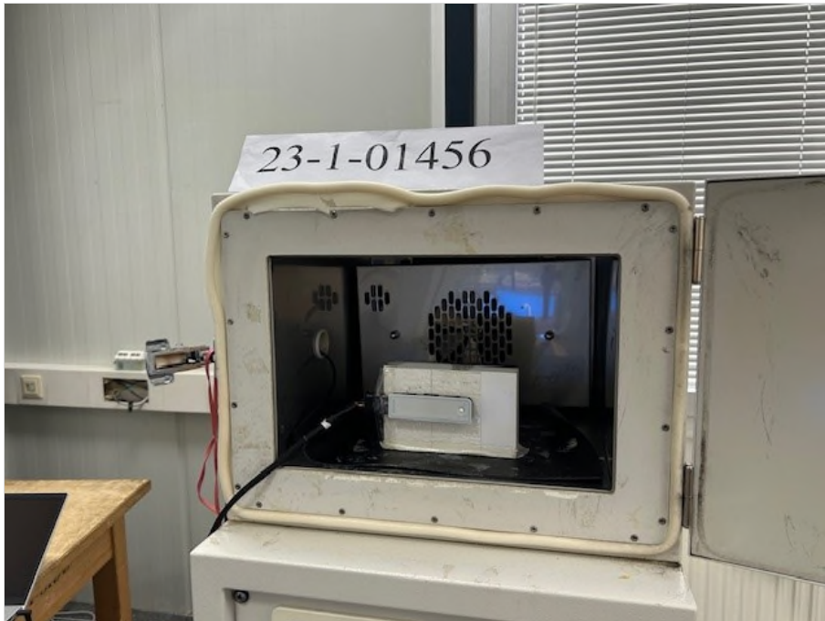
Photograph 9: EUT test setup extreme condition tests, close up view_EUT
