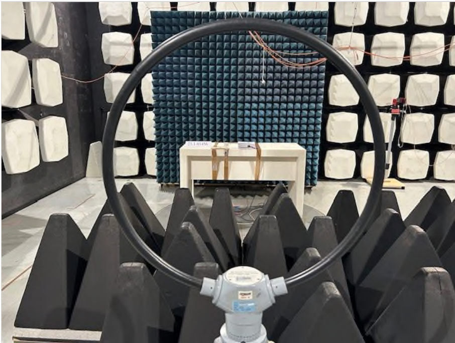
Photograph 1: EUT setup measurement ( f < 30\text{MHz} ), overview
