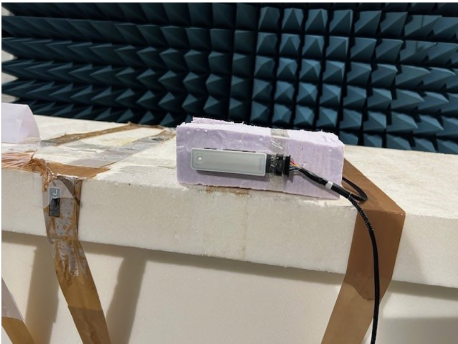
Photograph 2: EUT setup ( f < 30\text{MHz} ), close view overview
