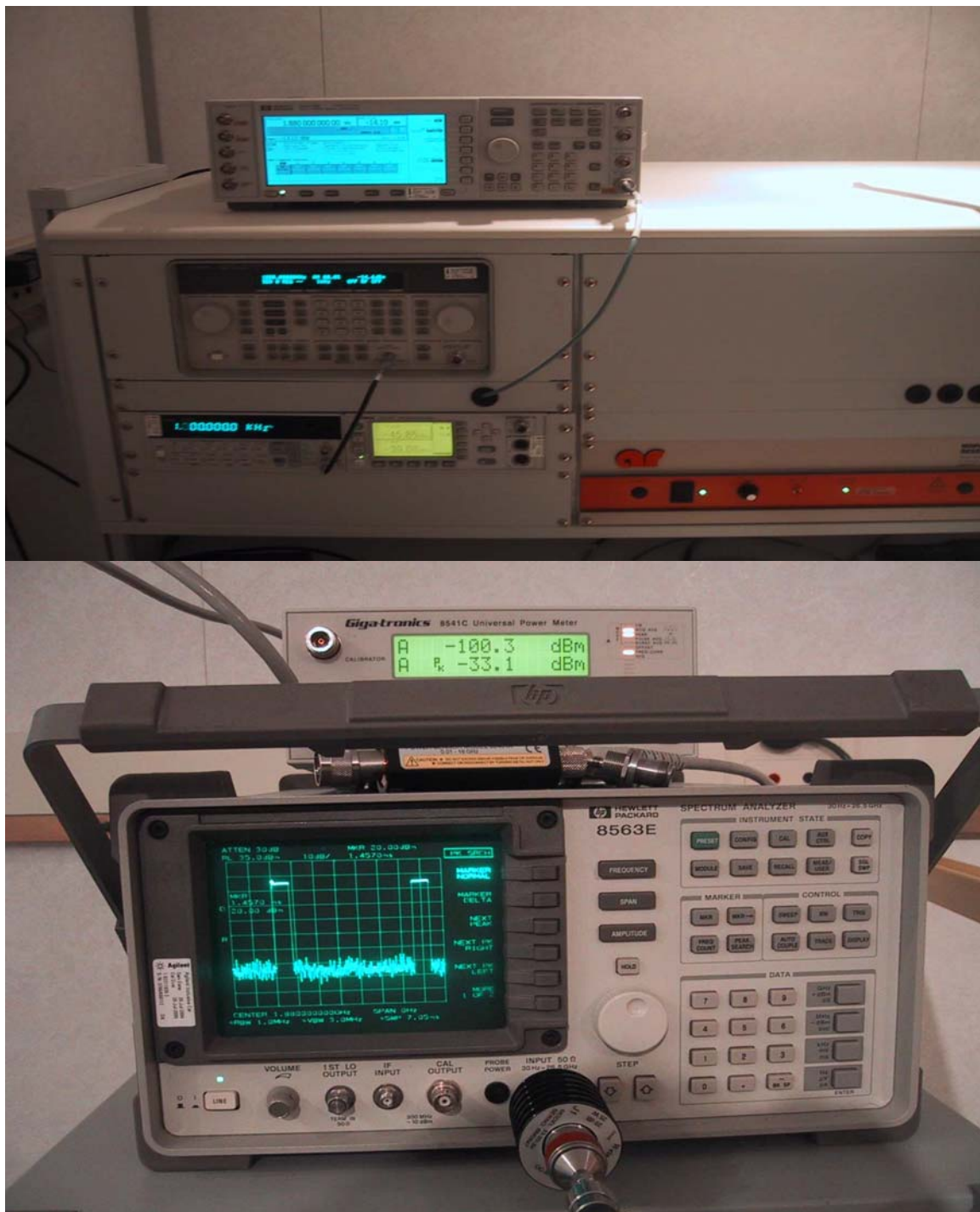
Figure 3 – Dipole validation and modulation measurement setup 2
