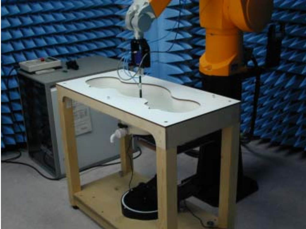
Fig.2 Photograph of the SAR measurement System
