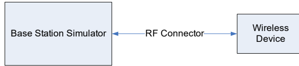
Figure 9-3 Power Measurement Setup
