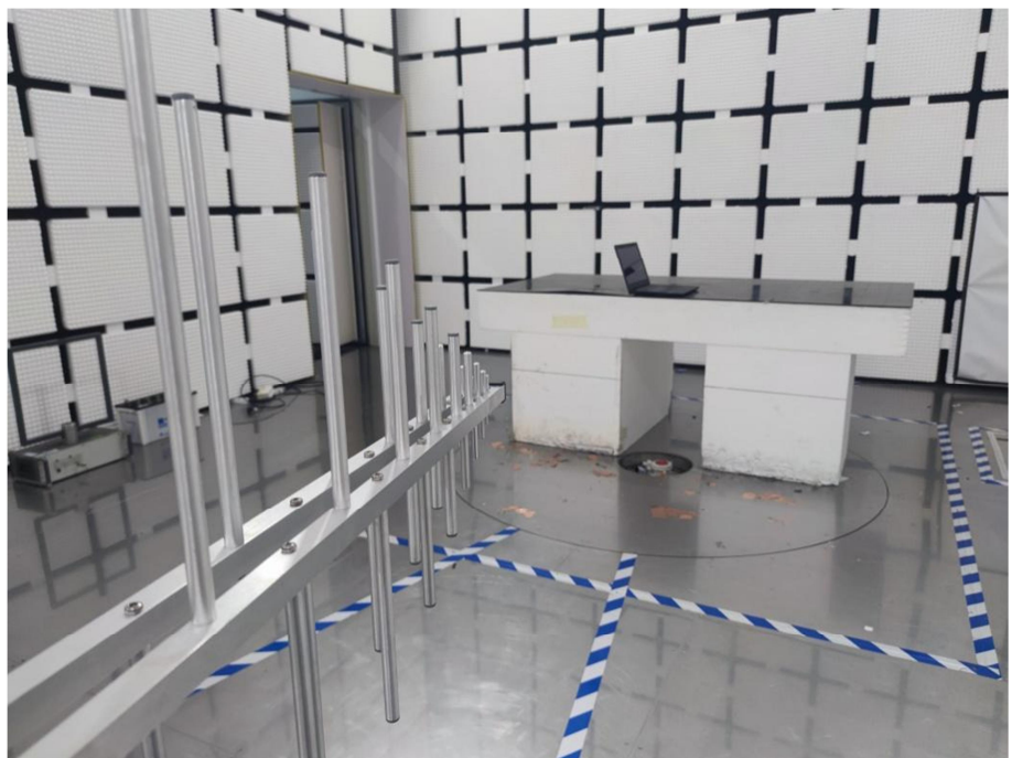
Radiation Emission Test Setup (30MHz to 1GHz)
