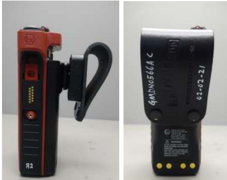
GMDN0566AC w/PMLN5004B with DUT: Side and back views (left to right)
