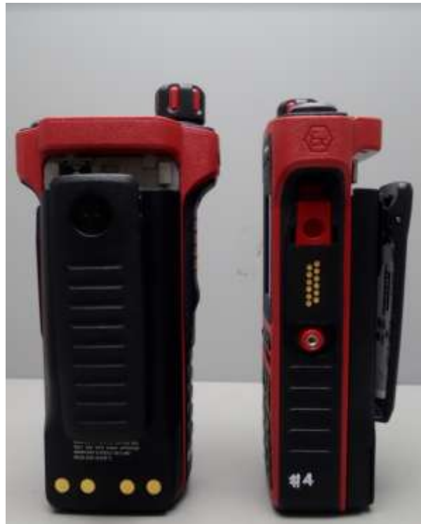
PMLN6086A with DUT: Back and side views (left to right)
