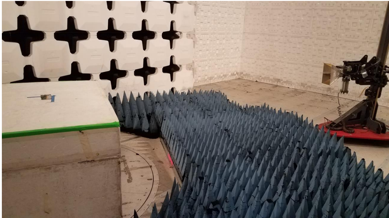
Figure 5. Radiated Emission Test Setup, 1 GHz to 18 GHz
