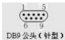
Figure 4. RS232 Pin Definition(Male/Needle Type)
