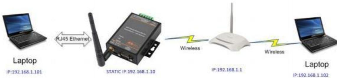
Figure 22. Ethernet Port Function(Bridge)
