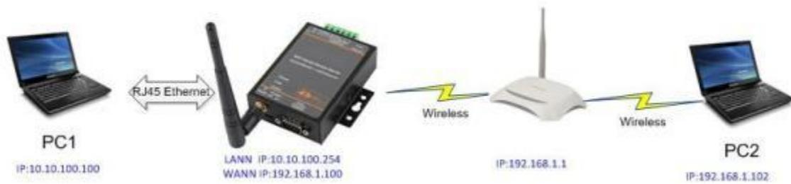
Figure 21. Ethernet Interface Function(Router)
