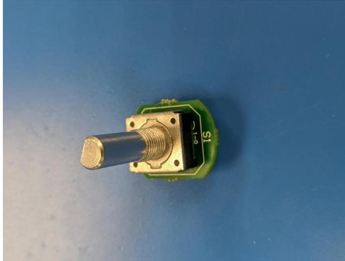
Figure 5: Encoder PCB – Top
