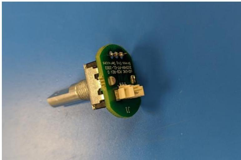
Figure 6: Encoder PCB – Bottom
