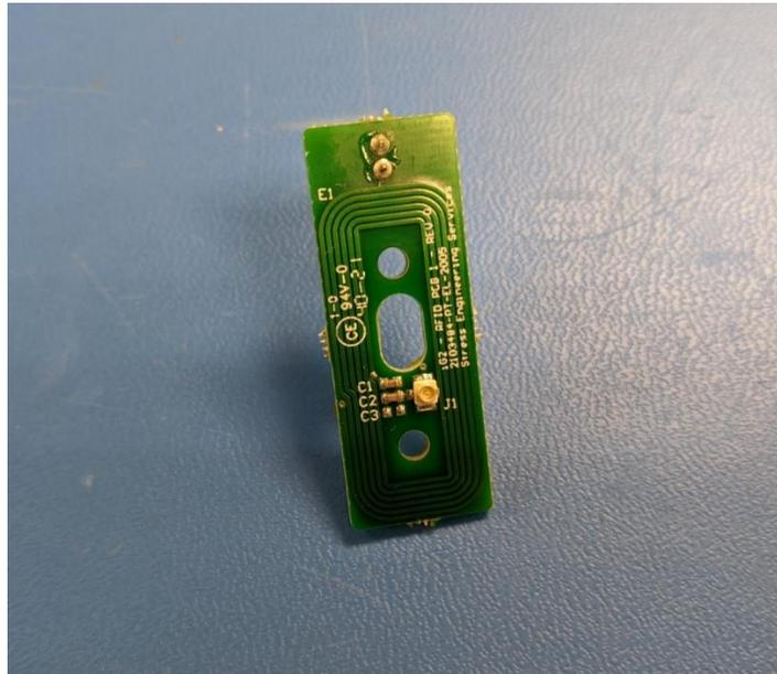
Figure 4: RFID PCB - Top
