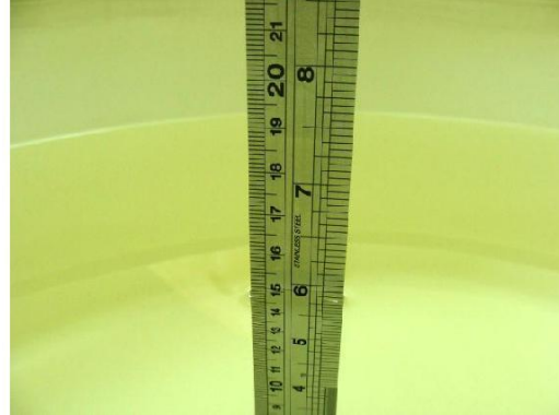
Fig 7.2 Photo of Liquid Height for Body SAR
